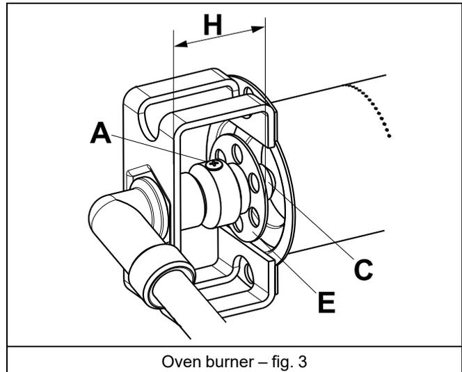
The primary air is correctly adjusted when the flame does not float with the burner cold and there is no flareback with the burner hot.
