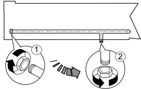
After installation, use soapy water to check connections for leaks.
